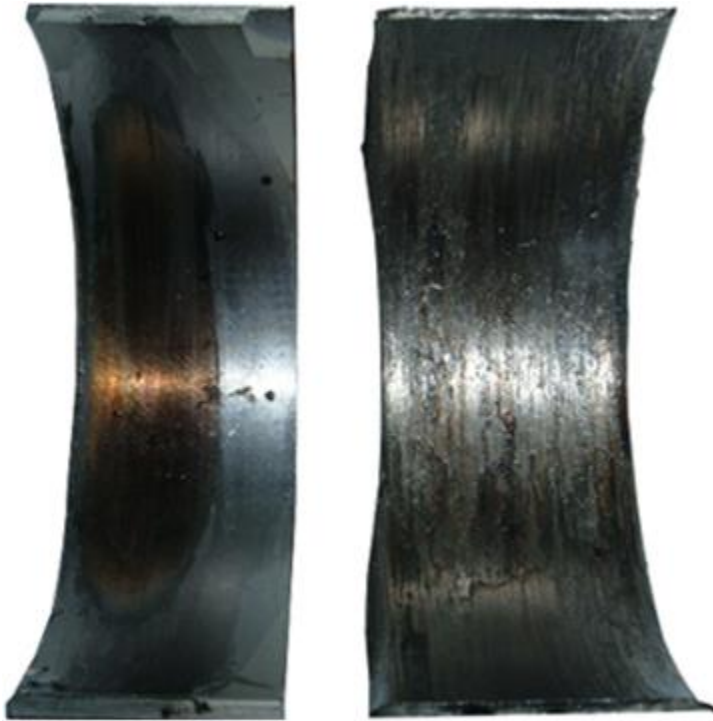
Fig.1 Bearings failed due to oil starvation
